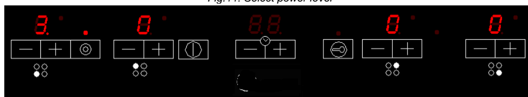
Fig.12: Heat Up function activated
