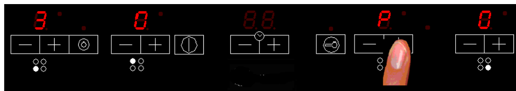
Fig. 4: Selected Booster function for a heater.
