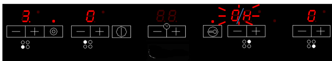
Fig. 15: Residual Heat (Cooktop On)
