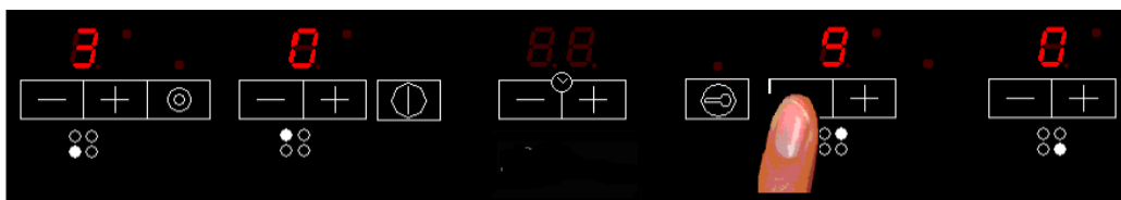
Fig. 5: Cancelling Booster function for a heater.
